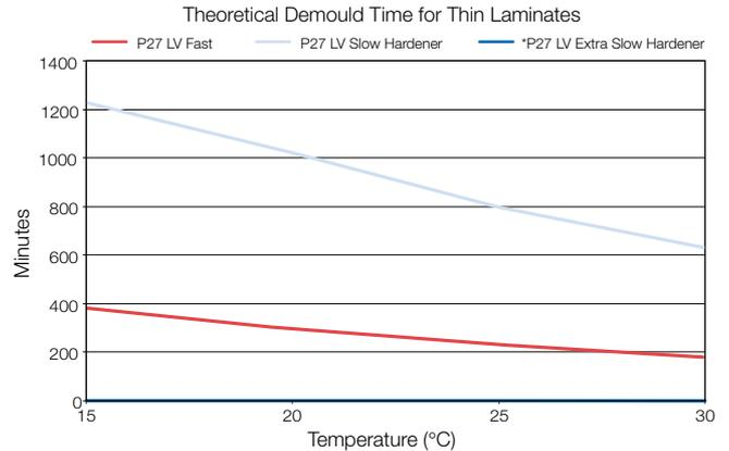
\*This hardener requires an elevated temperature cure – demould times at temperatures of 15-30°C are not recommended.
